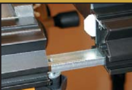
Close-up of Steel Guide Pin engaging SawTrain Rail.
