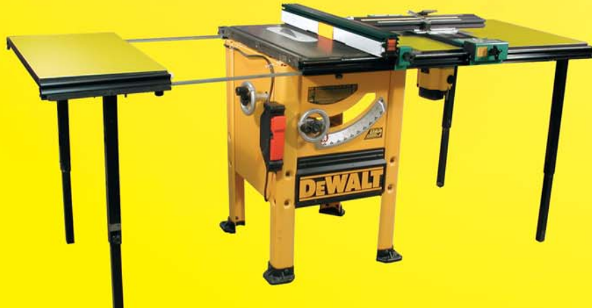
SEB-32 Extender Bars used to extend range of Floating Table.
